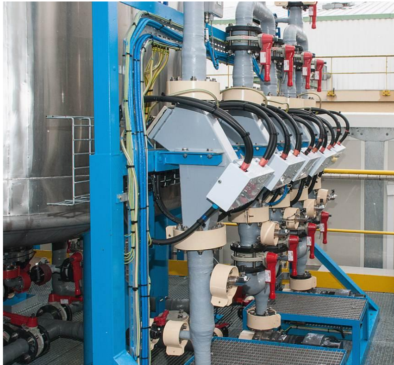
Industrial electrodes installed on a SOFHYS treatment unit (chemical industry)
